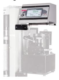
The HCM-5090 is a manually-operated digital indicator that provides many of the features of the HCM-5070 and HCM-5080 digital controllers, such as pre-programmed standards and data acquisition capabilities.
