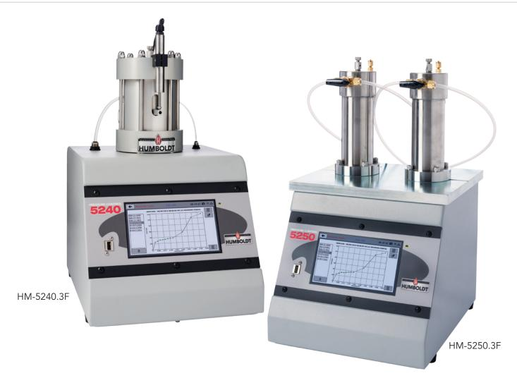
The HM-5240.3F and HM-5250.3F triaxial-specific pressure controllers are designed specifically for geotechnical laboratory triaxial testing, such as Unconsolidated Undrained, Consolidated Undrained and Consolidated Drained tests. Both pressure controllers provide control and monitoring of cell pressure, back pressure, pore water measurement and volume change when used with Humboldt's elite series load frames.
