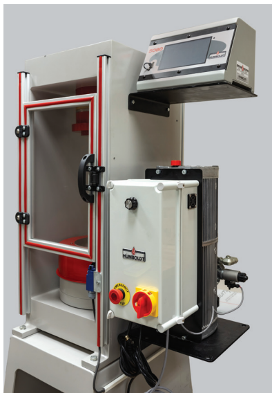
Photo #6— Controller and Pump mounted to Compression Machine
