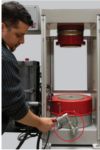
Photo #8— connecting the hydraulic hose to the compression machine
