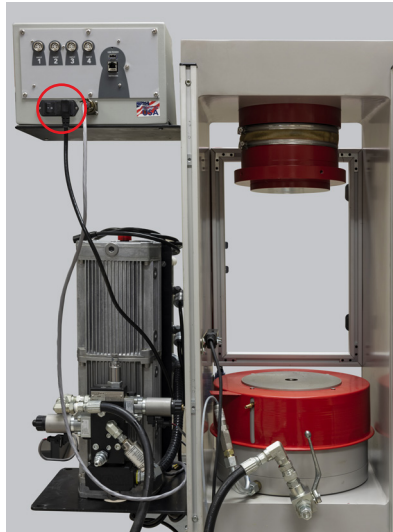
Photo #12— connecting AC hookup from the pump controller to the HCM-5080 controller.
