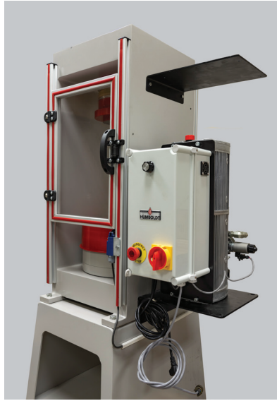
Photo #4— mounting controller bracket
