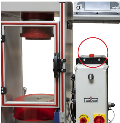
Photo #9— Location of red oil cap, which needs to be removed.
