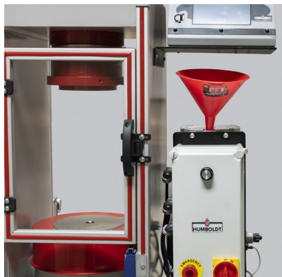
Photo #10— Fill pump with hydraulic oil.
