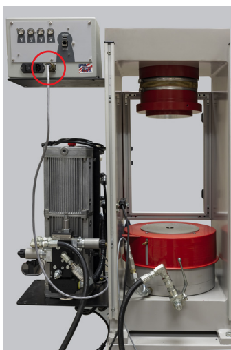
Photo #11— connecting the pump controller to the HCM-5080 controller.
