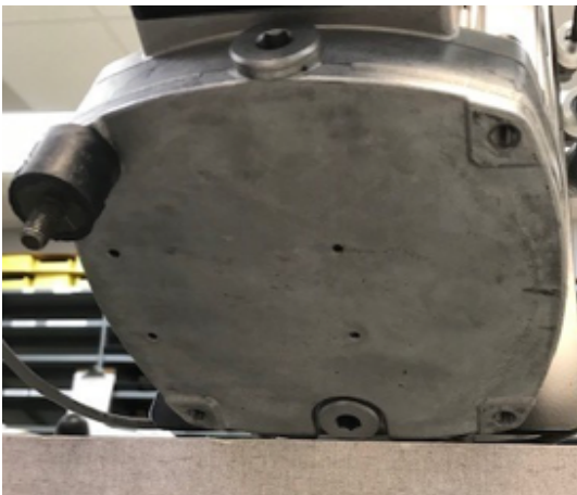
Photo #2— Installing rubber shock spacers
