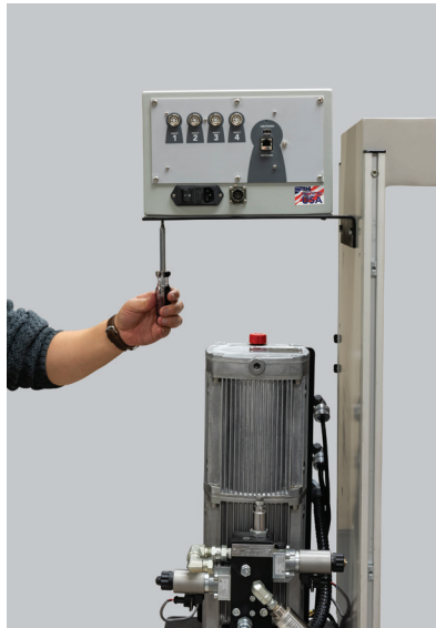
Photo #5— attaching controller to support bracket
