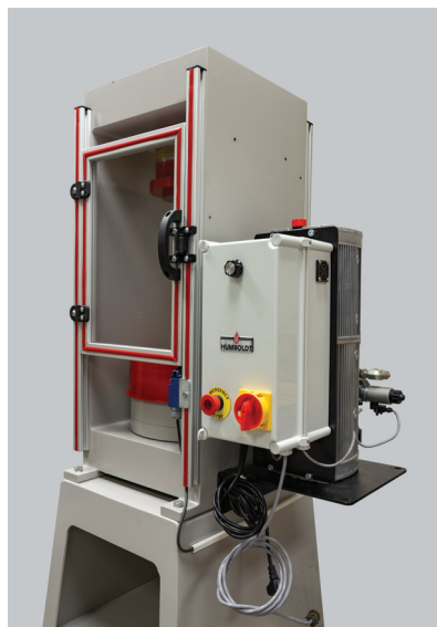
Photo #3— Pump mounted to support bracket
