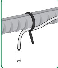
Secure the cable and temperature probe below the rebar
