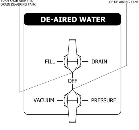
FIGURE 2 DE-AIRING TANK CONTROL VALVES
