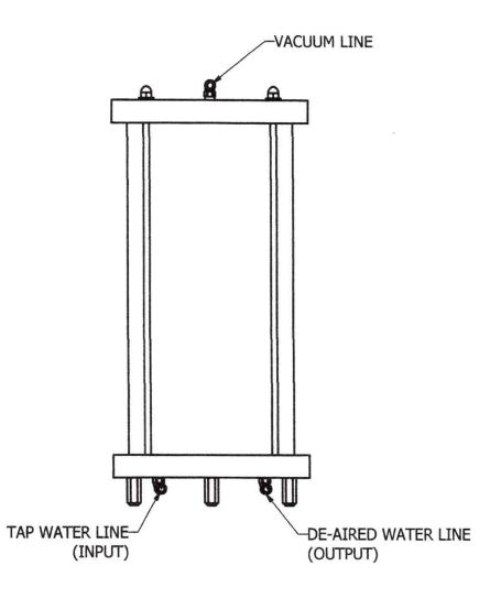
FIGURE 1 HM-4187H AIR AND WATER CONNECTIONS
