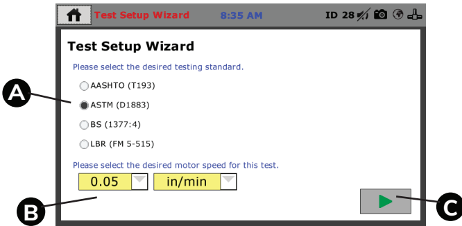
Figure 26: CBR / LBR Test Setup
