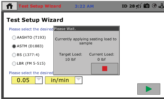
Figure 29: Applying Seating Load
