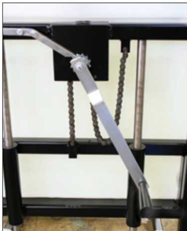
Crank for raising and lowering the shelf showing safety stop device.
