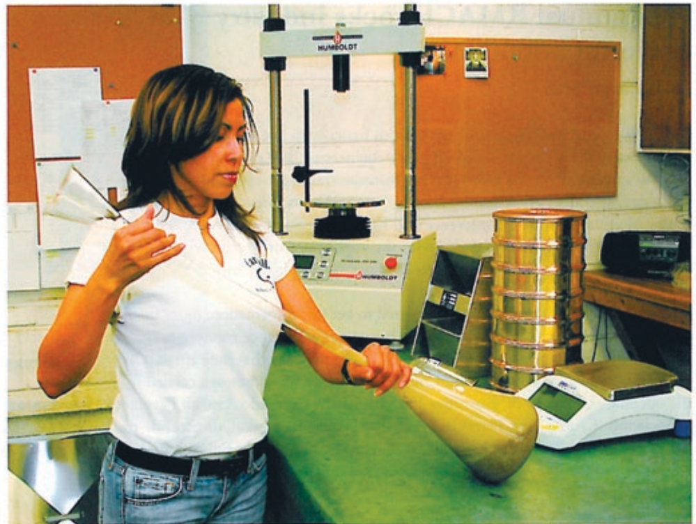
When performing bulk specific gravity tests, lab techs eliminate all released air during the soak period before taking final readings. The flask must be completely shaken and agitated, and then allowed to rest undisturbed so all of the air has escaped.
