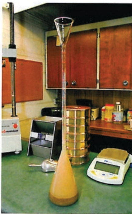
The Phunque flask can be used to double-check the specific gravity of incoming aggregate to ensure you've got what you need to make a spec-perfect mix.
