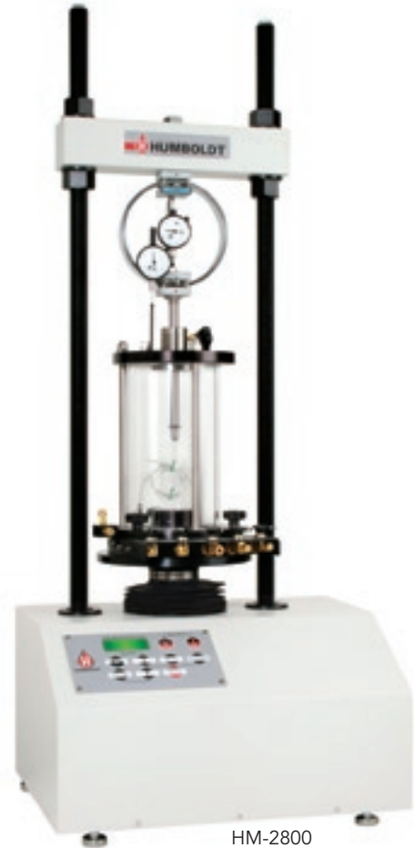
HM-2800 w/ typical Triaxial Setup
