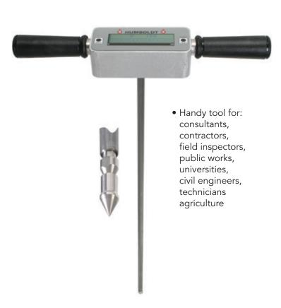
Humboldt's HS-4210 Digital, Static Cone Penetrometer (DSCP), with its large, digital readout, makes testing and recording readings easy. The DSCP can be used to evaluate soil consistency by determining the soil's level of compaction and/or the bearing capacity. The DSCP is especially useful in evaluating shallow foundations and pavement subgrades where fine-grained and soft soils are being used.
