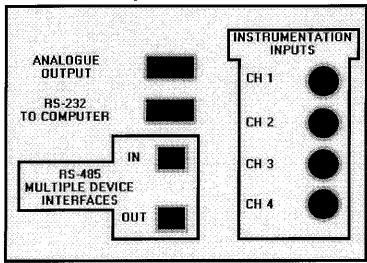
Connect the appropriate transducers to the sockets marked CH1, CH2, CH3, & CH4. The following pin out is used for connections:
