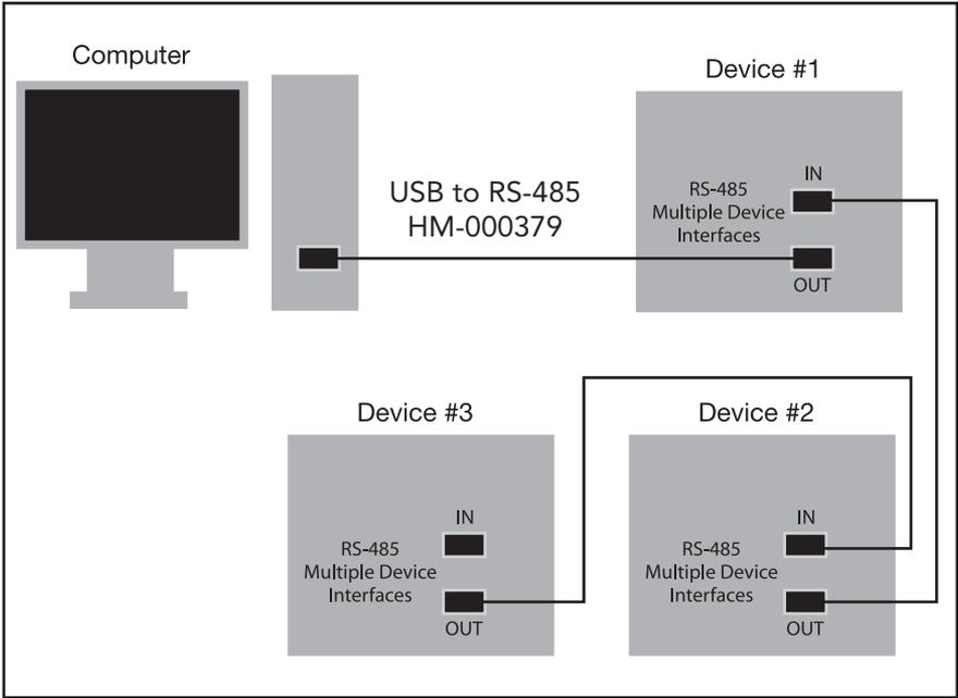
Figure 4. Diagram illustrating computer and multiple device connections.
