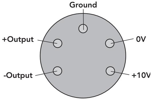
Figure 1. Compatibility wiring diagram for 3rd party cables
