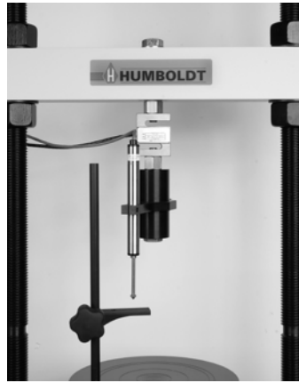
Figure 5. UU Triaxial Setup
