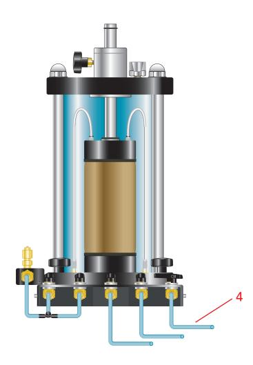
4. Connect the tubing from the Top Burette Assembly on the pressure panel to the Top Input on the right-hand side of the Triaxial cell.
