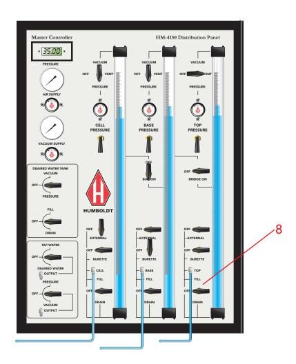
8. Turn the Top Pressure Burette assembly's Fill/Drain valve to the off position.
