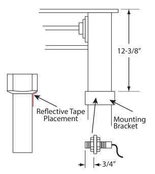
From the front, observe the clamping plates clamped by a hand knob to the right side beam. The retro-reflective, infra-red sensor is mounted in front and secured with two nuts, one on each side.
