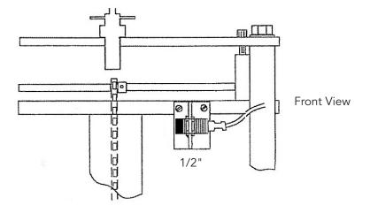
**H-1334BA** — Installing the Proximity Sensor for your H-1334BA Automatic Counter on a Humboldt H-1364, H-1366 Marshall Compactor.
