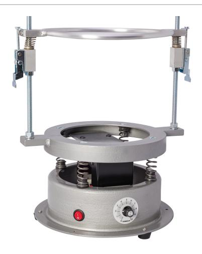
Vibrating, De-airing Device
