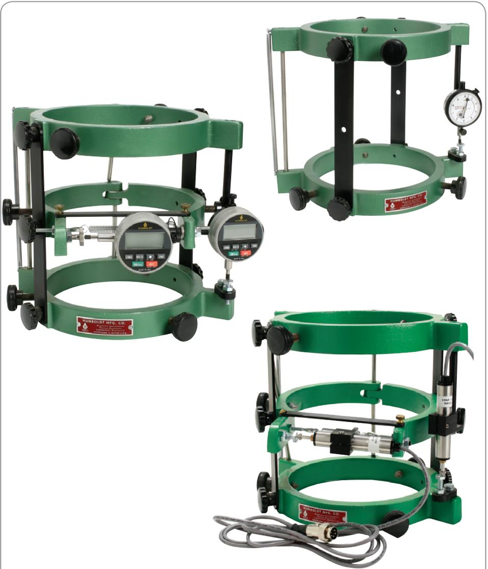
Compressometers / Extensometers
