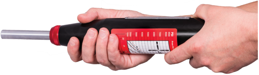
Figure 3: Push the piston in as far as it will go
