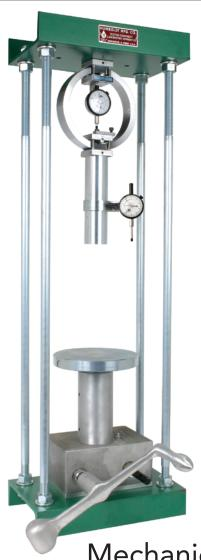
Mechanical Loading Press for CBR
