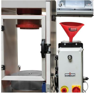
Photo #10— Fill pump with hydraulic oil.
