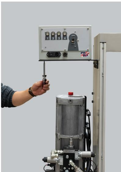
Photo #5— attaching controller to support bracket
