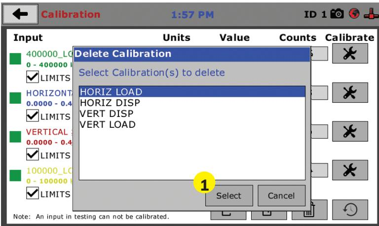
On this screen select an Input calibration to delete, one at a time, and then press the Select button **(1)**. The calibration will be deleted. You can do this for all Inputs you wish to calibrate.
