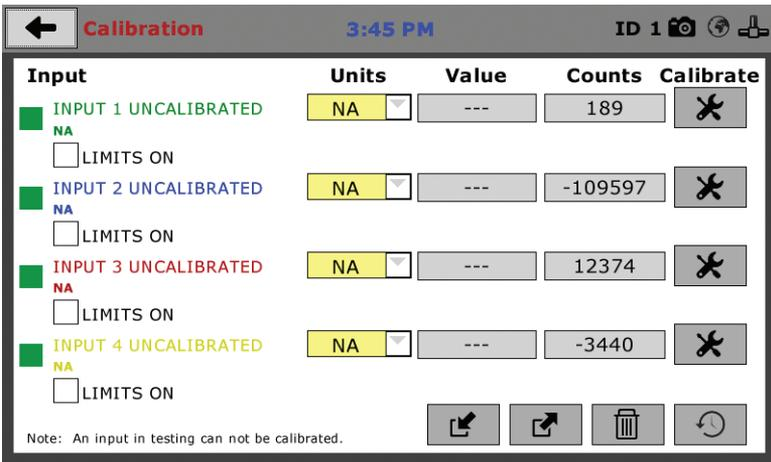
Calibrating your instrumentation to the appropriate Input requires a separate device, which can provide precise and specific loads or displacement, and, which has been certified to be accurate. The calibration process involves plugging the instrumentation into the HCM-5090 while placing the instrumentation into the certified calibration device, which provides a specific set load or displacement.
