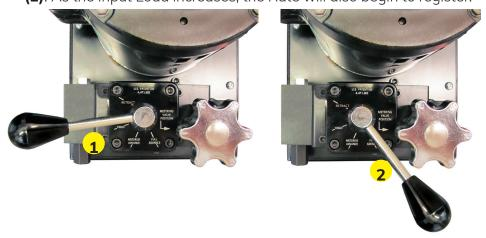
Continue with the Hydraulic Load Control Valve in the Full Advance position until you reach a reading that is 40% of the Anticipated Break Value. In our example that would be 4000 psi/sec, which is 40% of our Anticipated Break Value of 10000 psi/sec (1), see below.
