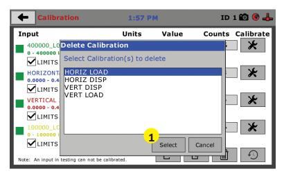
On this screen select an Input calibration to delete, one at a time, and then press the Select button **(1)**. The calibration will be deleted. You can do this for all Inputs you wish to calibrate.
