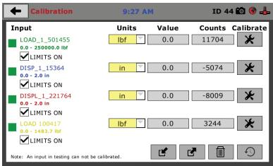
The screen above shows a typical calibration setup. In this example, the HCM-5090 has been set up with two channels for Load and two channels for Displacement.
