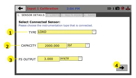
On Tab 1, the Sensor Type **(1)** will default to Load. For Capacity **(2)**, fill in the maximum capacity of the sensor and choose either lbf, kN, N or kgf. For FS output **(3)**, refer to the calibration sheet, which came with the instrument your are using and enter it here and then choose mV/V. The next page shows typical calibration sheets with the FS Output information highlighted in orange.
