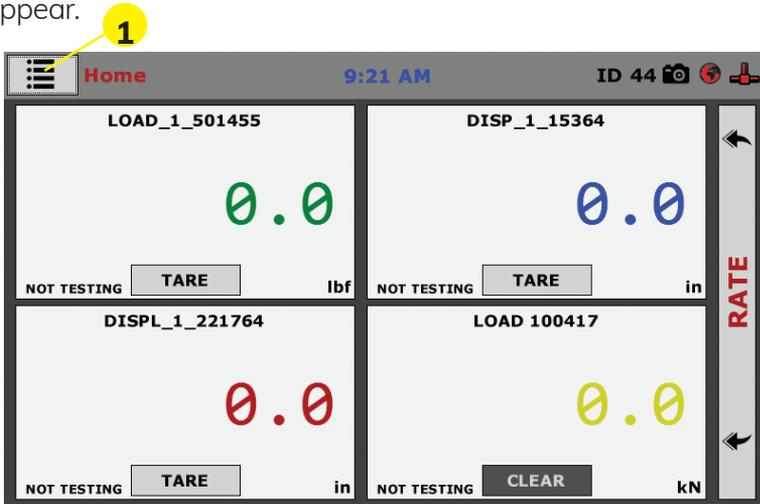
From this screen, to confirm your machine instrumentation has been calibrated or to begin the calibration process, navigate to the Calibration section by clicking the Menu icon in the top left corner of the screen (1). When you click on this button, you will see a drop-down menu appear, see below.
