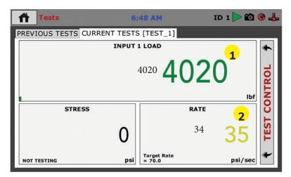
Once the Load reaches the 40% reading, switch the Hydraulic Load Control Value to the Metered Advance position (3) for the remainder of the test (See below). You will want to use the hydraulic valve on the compression machine pump (4), (see below), to adjust the Rate in the Rate section (2) of the Test window (see above) so that it reads  $35 \pm 7$  psi/sec.
