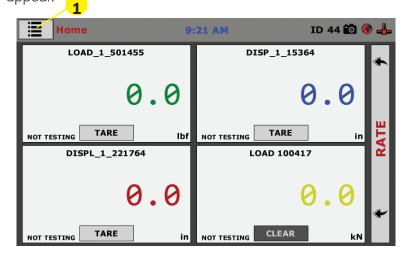
From this screen, to confirm your machine instrumentation has been calibrated or to begin the calibration process, navigate to the Calibration section by clicking the Menu icon in the top left corner of the screen (1). When you click on this button, you will see a drop-down menu appear, see below.
