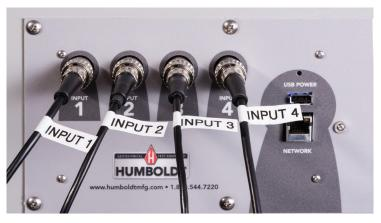
If you purchased multiple compression machines and/or compressometers/extensometers with your Compression machine/Digital Indicator, their input plugs will be marked to correspond
