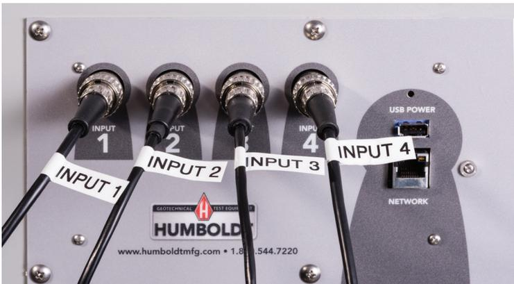
If you purchased multiple compression machines and/or compressometers/extensometers with your Compression machine/Digital Indicator, their input plugs will be marked to correspond
