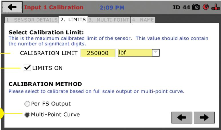
On Tab 2, in the Calibration Limit field (1), enter the maximum calibrated limit of the sensor. This value should contain the number of decimal points you require for degree of accuracy, up to 5 points. Limits On (2), has no bearing on operation with the HCM-5090. Calibration Method (3) determines whether this calibration will be based only on the maximum load capacity of the sensor or upon a multi-point curve of up to a maximum of 10 points.
