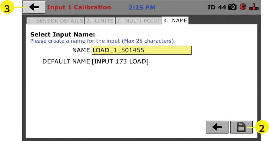
On Tab 4, you will be asked to name the calibrated Input. Fill in your Input Name and click on the Save button **(2)** to save your calibration.
