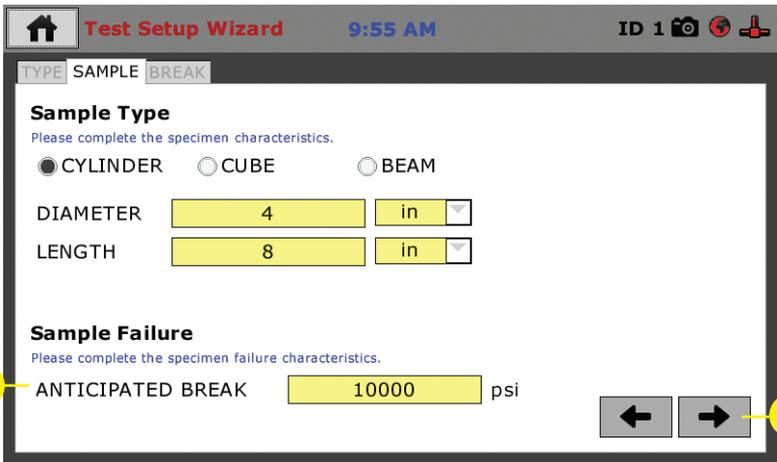
You can also provide an Anticipated Break (Sample Failure) value in the yellow field **(3)** provided.
