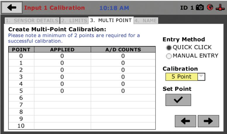
On Tab 3 you will be able to set the number of points you want to use for your calibration. You can choose 1-point, 5-point, 10-point or Custom, which allows you to use any number of points up to a total of 10. In the example on the previous screen shot above, a 5-point calibration has been chosen.
