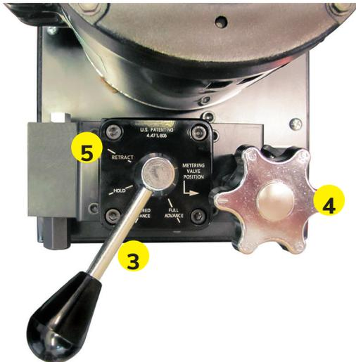
When the specimen breaks, the Digital Indicator will continue to log until it detects a reduction in the Load of 10% of the Peak Value. At this point it will automatically stop logging. At this point, move the Hydraulic Load Control Valve to the Retract position **(5)**.
