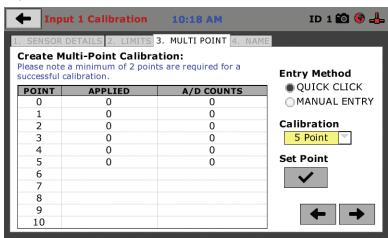
On Tab 3 you will be able to set the number of points you want to use for your calibration. You can choose 1-point, 5-point, 10-point or Custom, which allows you to use any number of points up to a total of 10. In the example on the previous screen shot above, a 5-point calibration has been chosen.
