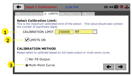
On Tab 2, in the Calibration Limit field **(1)**, enter the maximum calibrated limit of the sensor. This value should contain the number of decimal points you require for degree of accuracy, up to 5 points. Limits On **(2)**, has no bearing on operation with the HCM-5090. Calibration Method **(3)** determines whether this calibration will be based only on the maximum load capacity of the sensor or upon a multi-point curve of up to a maximum of 10 points.
