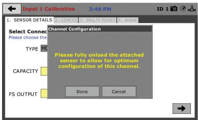
If you choose Multi-Point (Recommended calibration method) Curve and click on the Right Arrow in the bottom right-hand corner of the screen, you will be taken to Tab 3.
