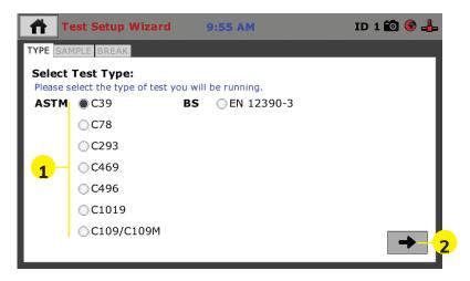
Select a test **(1)** from the choices provided on the screen by clicking on the radio button next to the test. In this example we have chosen ASTM C39. Then, click on the Right Arrow button **(2)** in the bottom right-hand corner.
