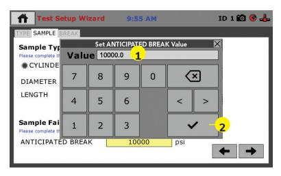
Once you have entered a value, Click the Check Mark **(2)** in the lower right-hand corner to save the value. You will be returned to the Sample Tab of the Test Setup Wizard.
