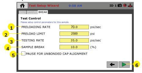
On this screen, you will enter values, which dictate your test parameters. To begin, you can set a Preloading Rate (1) and Limit (2), which establishes a base load prior to the actual test.
