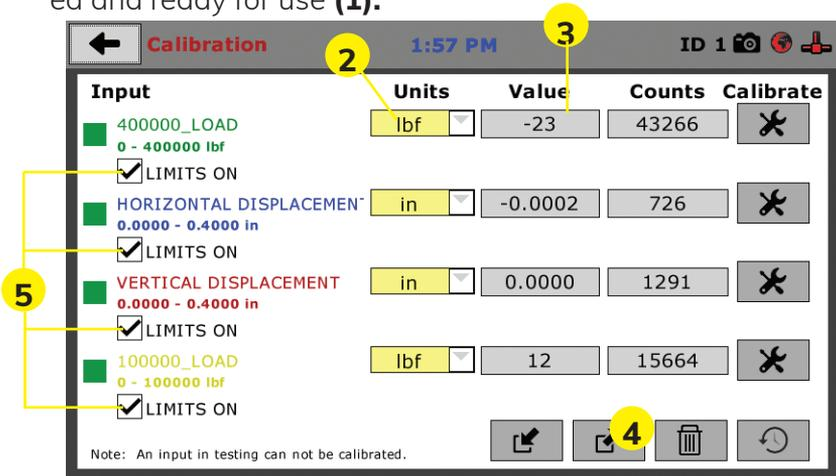
Each channel has a “Limits On” check box. Use the Limits On to keep the machine from exceeding the sensor limits of the instrumentation. By selecting this option, before the test can exceed the limits of the sensors, all tests will stop running and the motor will stop to avoid damaging connected instrumentation.
