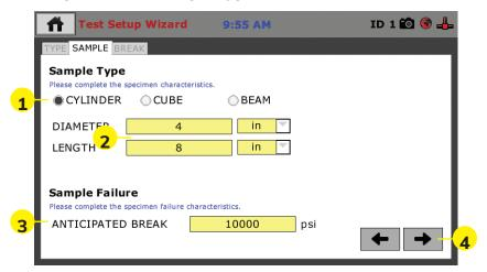
The screen above allows you to choose the type of test specimen (1) to be tested and to fill in its size in the corresponding yellow fields (2). Because we chose ASTM C39 on the previous screen, the machine will automatically choose Cylinder as your Sample Type. When you click on the yellow fields, a Set Value screen will popup to allow you to set these values, see below (1). Once you have entered a value, Click the Check Mark (2) in the lower right-hand corner to save the value, see below.
