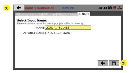
On Tab 4, you will be asked to name the calibrated Input. Fill in your Input Name and click on the Save button (2) to save your calibration.
