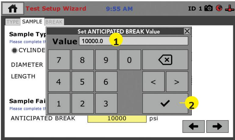
Once you have entered a value, Click the Check Mark **(2)** in the lower right-hand corner to save the value. You will be returned to the Sample Tab of the Test Setup Wizard.
