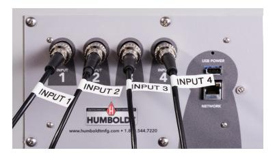
If you purchased multiple compression machines and/or compressometers/extensiometers with your Compression machine/Digital Indicator, their input plugs will be marked to correspond to the correct type of input on the back of the Digital Indicator. Remember: Inputs 1 and 4 are configured to read Load and Inputs 2 and 3 are configured to read Displacement.
