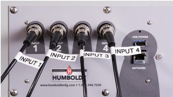
If you purchased multiple compression machines and/or compressometers/extensometers with your Compression machine/Digital Indicator, their input plugs will be marked to correspond to the correct type of input on the back of the Digital Indicator. Remember: Inputs 1 and 4 are configured to read Load and Inputs 2 and 3 are configured to read Displacement.
