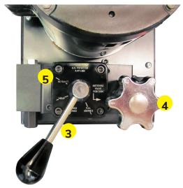
When the specimen breaks, the Digital Indicator will continue to log until it detects a reduction in the Load of 10% of the Peak Value. At this point it will automatically stop logging. At this point, move the Hydraulic Load Control Valve to the Retract position (**5**).
