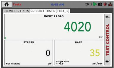
At this point, see below, move the Hydraulic Load Control Valve from the Hold position (1) to the Full Advance position (valve fully open) (2). As the Input Load increases, the Rate will also begin to register.
