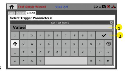
In the Value Field **(1)** (above) give your test a name. When finished, click on the check mark key **(2)** to save. Once saved, the Indicator will be ready to log, depending upon how you set your Start Parameters. You will see the following screen, ready to start logging.
