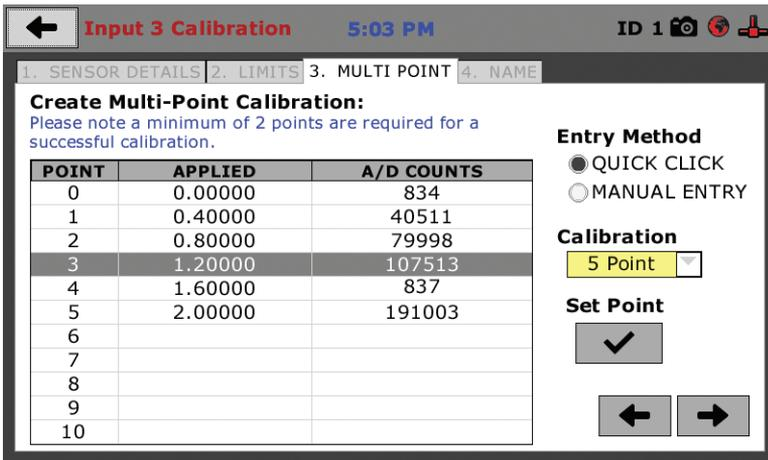
Each point would be chosen by clicking on the corresponding point row above. The load would be applied to the sensor and an A/D Counts reading would appear. To set the point, click on the Set Point button **(1)**. This would be repeated until all points have been set. In the example above, Point 3 is being calibrated and is ready to have the Set Point button **(1)** clicked. Point 4 still needs to be calibrated.
