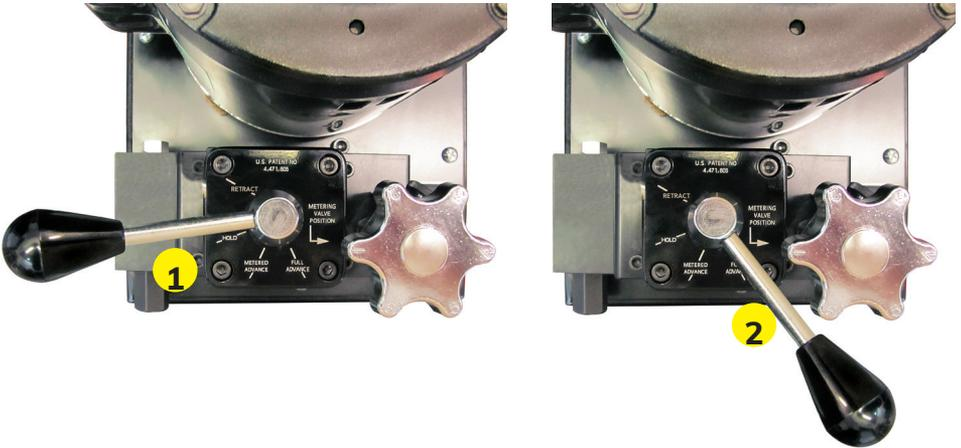
Continue with the Hydraulic Load Control Valve in the Full Advance position until you reach a reading that is 40% of the Anticipated Break Value. In our example that would be 4000 psi/sec, which is 40% of our Anticipated Break Value of 10000 psi/sec **(1)**, see below.
