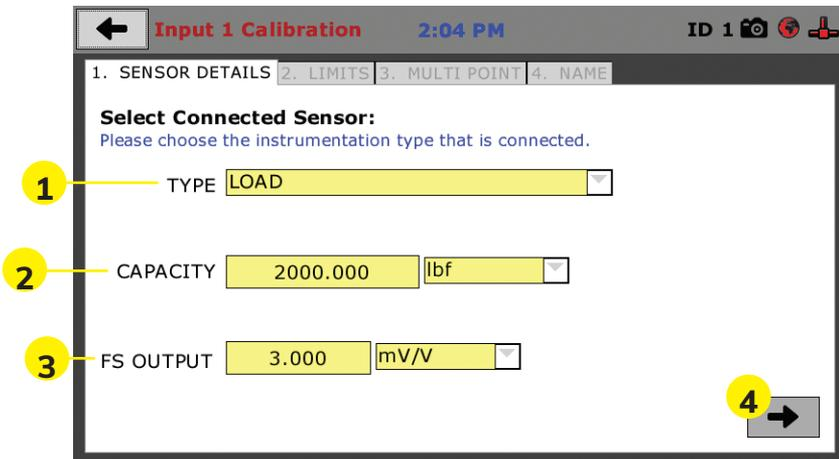
On Tab 1, the Sensor Type **(1)** will default to Load. For Capacity **(2)**, fill in the maximum capacity of the sensor and choose either lbf, kN, N or kgf. For FS output **(3)**, refer to the calibration sheet, which came with the instrument your are using and enter it here and then choose mV/V. The next page shows typical calibration sheets with the FS Output information highlighted in orange.
