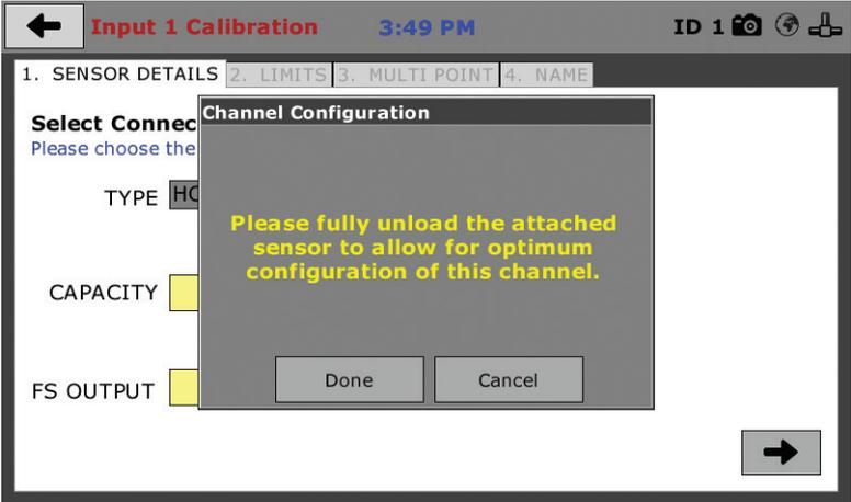
If you choose Multi-Point (Recommended calibration method) Curve and click on the Right Arrow in the bottom right-hand corner of the screen, you will be taken to Tab 3.
