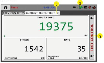
Clicking on this tab opens the Test Control panel, see below.
