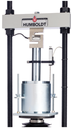
Figure #2 CBR Instrumentation Setup
