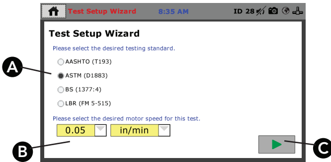
Figure 26: CBR / LBR Test Setup
