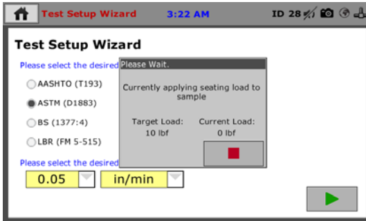
Figure 29: Applying Seating Load
