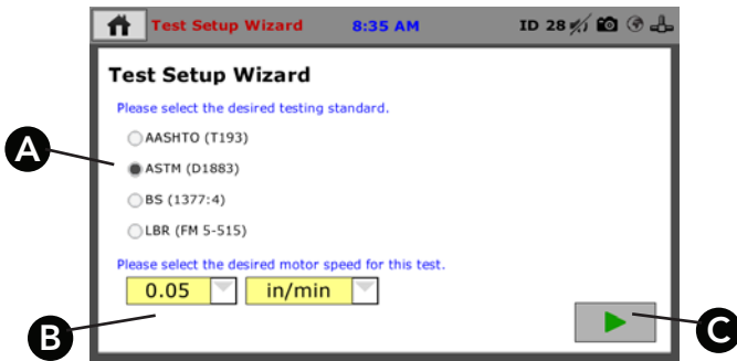
Figure 26: CBR / LBR Test Setup
