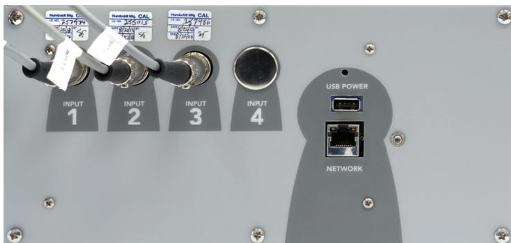
If you purchased multiple load cells and/or transducers with your machine, they will either be mounted and calibrated, or in the case of more than four (4) load cells/transducers, calibrated and assigned to a specific input, but not mounted.
