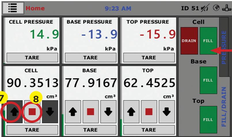
5. Select the Cell Fill Button **(6)** to allow water to flow from the water source to the Pressure Cylinder. When all air has been removed through the Bleed Valve and only clear water is exiting, close the Bleed Valve.
