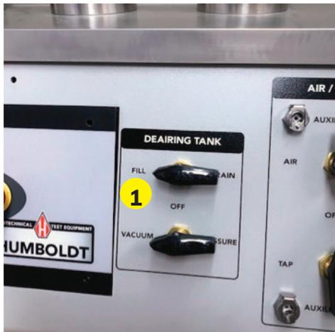
5. When the Deairing Tank is 3/4 full, turn the Deairing Tank FILL/DRAIN valve to the "OFF" position.
