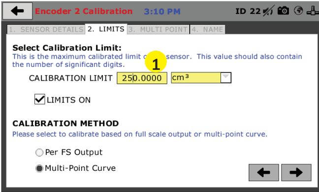
Ensure that the calibration limit is set to 250 cm<sup>3</sup> (1).
