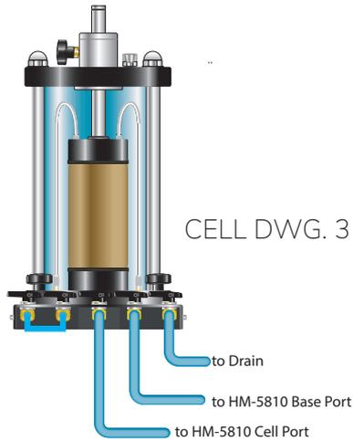
1. Ensure the Cell port on the Triaxial Cell is turned to OPEN.
