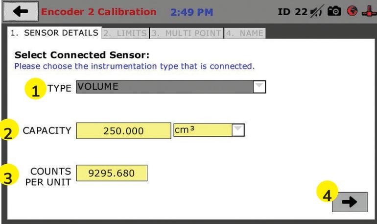
On Tab 1, the Sensor Type (1) will default to Volume. For Capacity (2), fill in the maximum capacity of the sensor and choose either lbf or kN.
