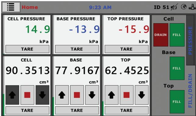
Ensure that the cell piston has been fully moved to the down position, you will then be prompted to reset encoder, select YES (1).
