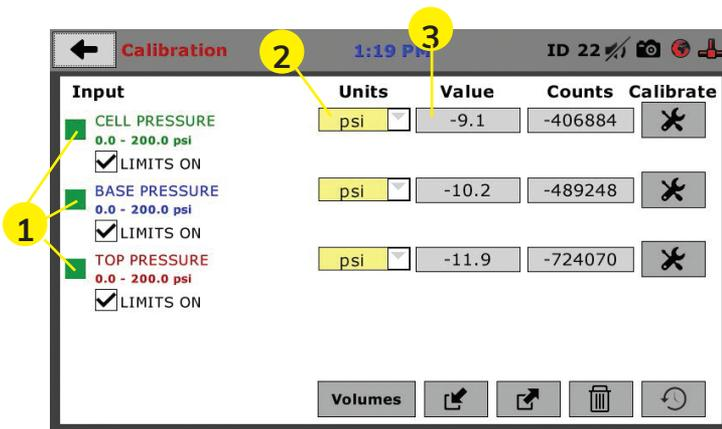
Each channel has a “Limits On” check box (1). Use the Limits On to keep the machine from exceeding the sensor limits of the instrumentation. By selecting this option, before the test can exceed the limits of the sensors, all tests will stop
