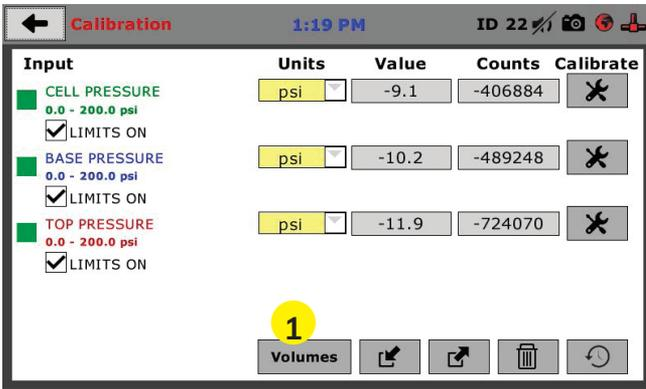
Now, we need to calibrate the Cell Volume. To get to the volumes calibration page you need to push the Volumes button at the bottom of the screen (1). However, calibration for volume on this is a bit different than what we are used to since it is based on a motor count rather than measuring the actual volume. In order to calibrate the volume the following steps have to be followed:
