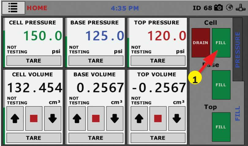
5. Once the Triaxial Cell is filled completely, turn the CELL VALVE on the Triaxial Cell to the OFF position (See CELL DWG. 2 below). Press the FILL tab on the touch screen to close the water supply.
