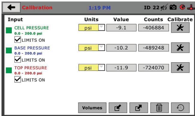
The screen above shows a typical cell pressure calibration setup. In this example, the HM-5810 has been set up for a standard Consolidated Drained or Undrained Triaxial setup. Input 1 is set up to read Cell Pressure of 0.0-200.0 psi; Input
