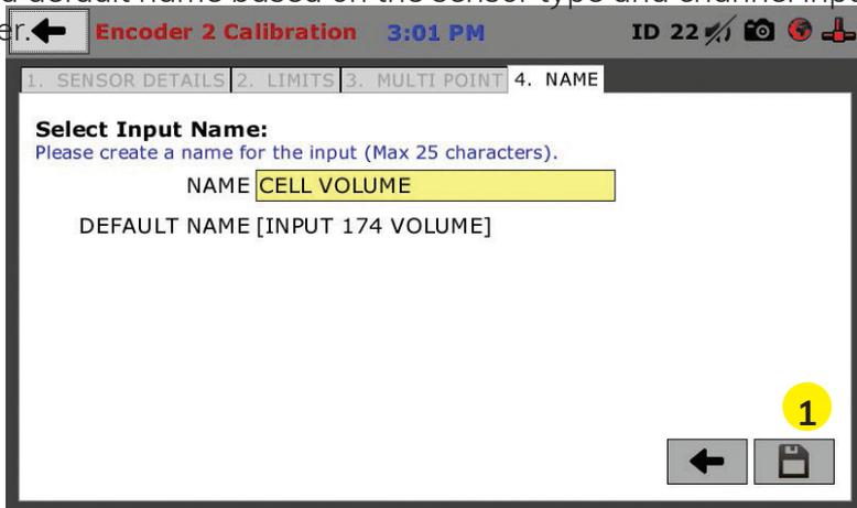
The screen will provide a default name, but you can name the Input anything you'd like. Once you've named the Input, click on the disk icon in the lower, right-hand corner **(1)**. This will save it. Use this method for calibrating any additional Inputs necessary.
