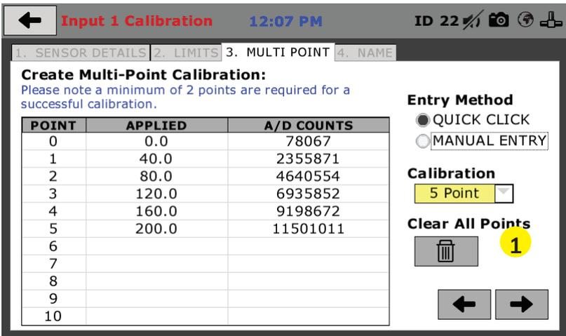
Each point would be chosen by clicking on the corresponding calibration point row. The load would be applied to the sensor and an A/D Counts reading would appear. To set the point, click on the Set Point button (1)
