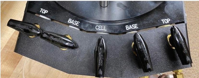
**NOTE:** If the Top port on the Triaxial cell was in the open position during the Saturation and Consolidation phases of the test the only step required is to apply a Top pressure that matches the current Base pressure.
