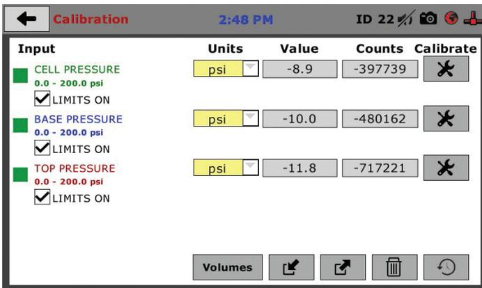
Calibrating your instrumentation to the appropriate Input requires a separate device, which can provide precise and specific loads or displacement, and, which has been certified to be accurate. The calibration process involves plugging the instrumentation into the HM-5810 while placing the instrumentation into the certified calibration device, which provides a specific set load or displacement.
