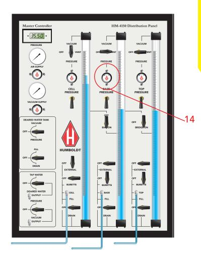
14. When the two pressures match, go back to the Base Pressure and increase it by 0.5 psi.
