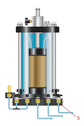
5. Loosen the nut holding the tubing on the Top Input valve of the Triaxial cell.
