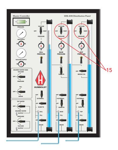
15. Turn the Base Pressure and the Top Pressure valves to Pressure position.
