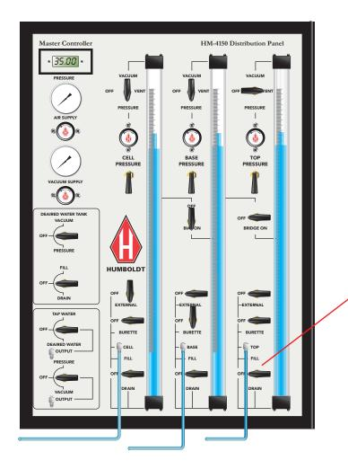
8. Turn the Top Pressure Burette assembly's Fill/Drain valve to the off position.
