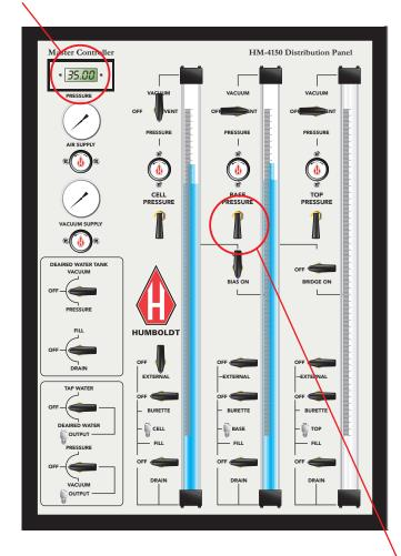
Flip this toggle up, which will reveal the Base Pressure in the Pressure window (12A) located at the top left corner of the HM-4150 Panel.
