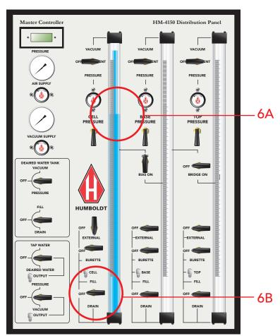
A. Slow the water II rate of the External Tube as the water level approaches this level.
