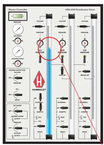
The water level in the Burette will adjust to the water level in the External Tube.
