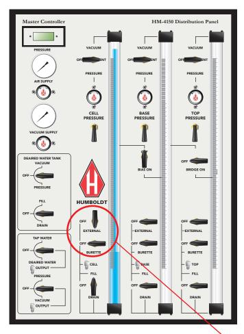
Turn the Burette Valve Indicator to the Off position and turn the External Valve Indicator to the On position (External).
