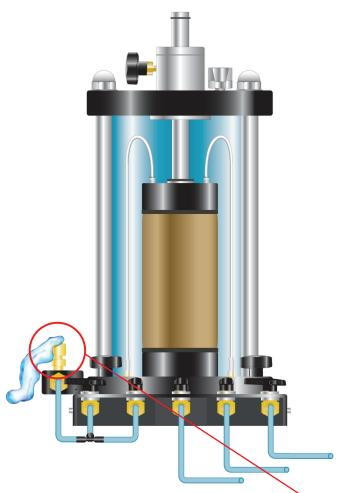
Open the Vent on the top of the De-airing Valve. Once water begins to flow out, close the Vent.
