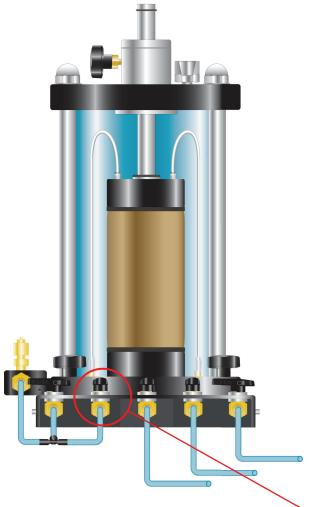
Open Base Valve located on the left-hand side of the Triaxial Cell.
