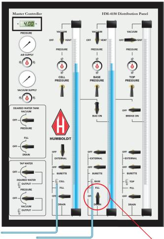
Turn Base Burette Assembly Fill/Drain Valve to Fill.
