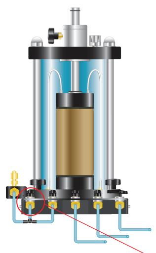
Open the Top Valve, located on the left-hand side of the Triaxial Cell.
