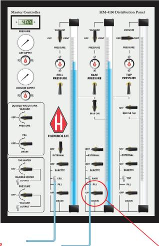
When air bubbles are no longer evident in the drainage line coming from the Cell.
