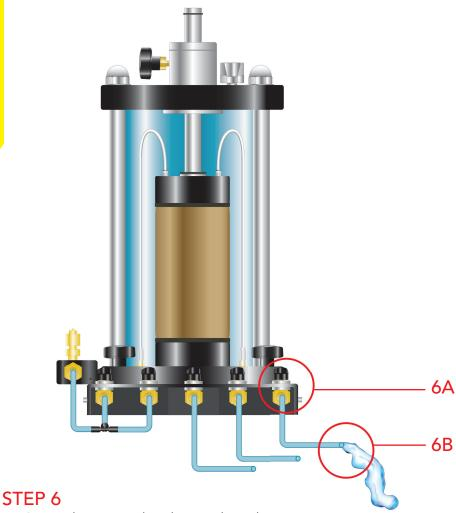
A. Open the Top Valve, located on the right-hand side of the Triaxial Cell.
