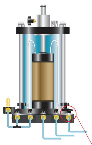
Then, close the Top Valve, located on the right-hand side of the Triaxial Cell.
