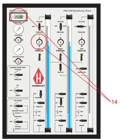
To check the resulting Cell Pressure in the Pressure window, flip the Base Pressure Toggle down and Flip the Cell Pressure toggle up. The Cell Pressure will be revealed. In this case, the Cell Pressure will read 33-35 psi (3-5 psi plus the next increment).
