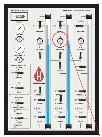
Adjust the Base Pressure Regulator to 20 psi.
