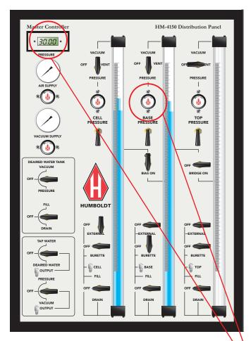
Flip the toggle below Base Pressure Regulator to the up position, then Adjust the Base Pressure Regulator to read 30 psi or to the next increment.
