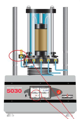
Record the Pore Pressure reading after approximately 1 minute.
