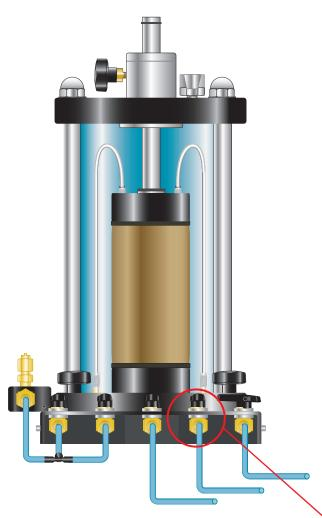
Open Base Valve located on the right-hand side of the Triaxial Cell.
