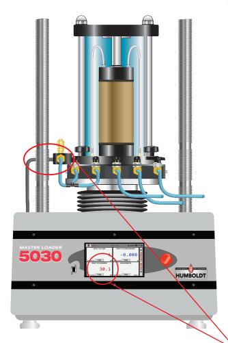
Readout of the Pressure Transducer should read approximately 30 psi.
