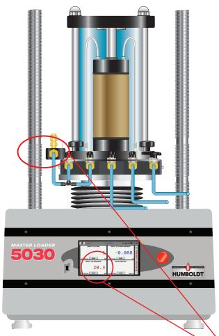
Check readout of Pressure Transducer attached to the De-airing Block on the Triaxial Cell. This should read approximately 20 psi.
