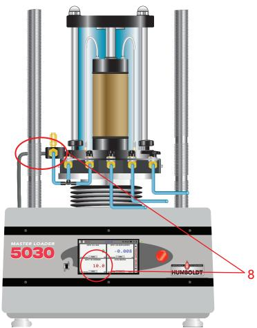
Check readout of Pressure Transducer attached to the De-airing Block on the Triaxial Cell. This should read approximately 10 psi.
