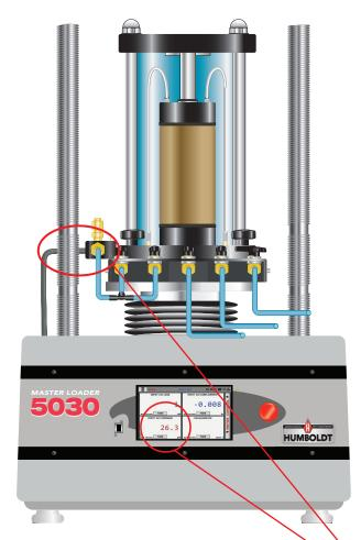
Record the Pore Pressure after approximately 2 minutes from the Pressure Transducer Readout.
