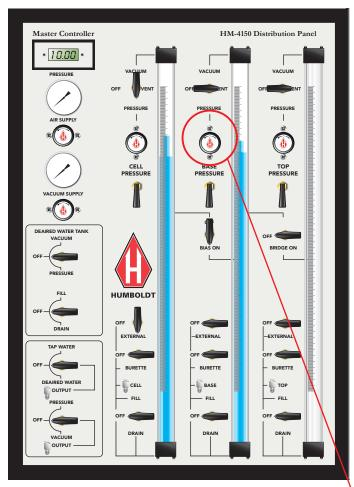
Adjust the Base Pressure Regulator to 10 psi.
