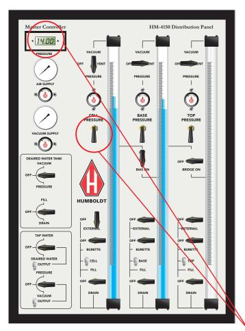
To check the resulting Cell Pressure in the Pressure window, flip the Base Pressure Toggle down and Flip the Cell Pressure toggle up. The Cell Pressure will be revealed.
