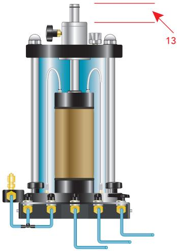
Measure Specimen reference height prior to Shear Stage.
