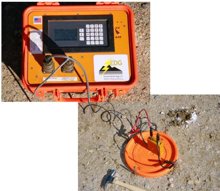
**Figure 44 Electrical density gauge testing used on the unbound materials.**
