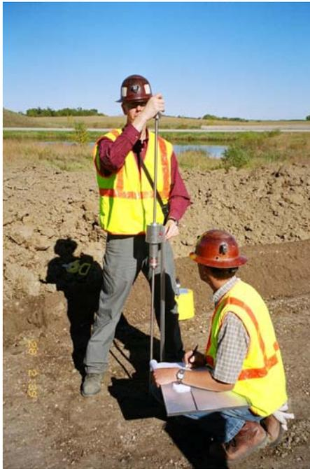
**Figure 26** Dynamic Cone Penetrometer testing to estimate the in situ shear strength of unbound materials (courtesy MnRoads).
