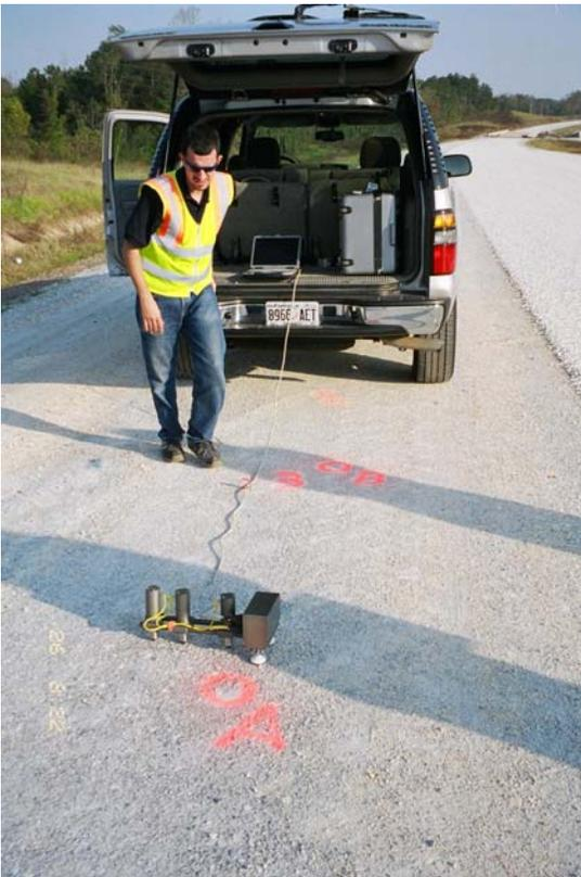
(b) Field testing using the DSPA.
