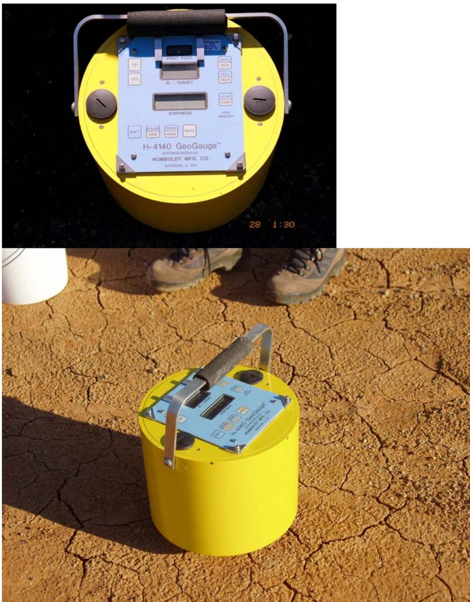
**Figure 35** GeoGauge used for stiffness testing on all unbound materials.
