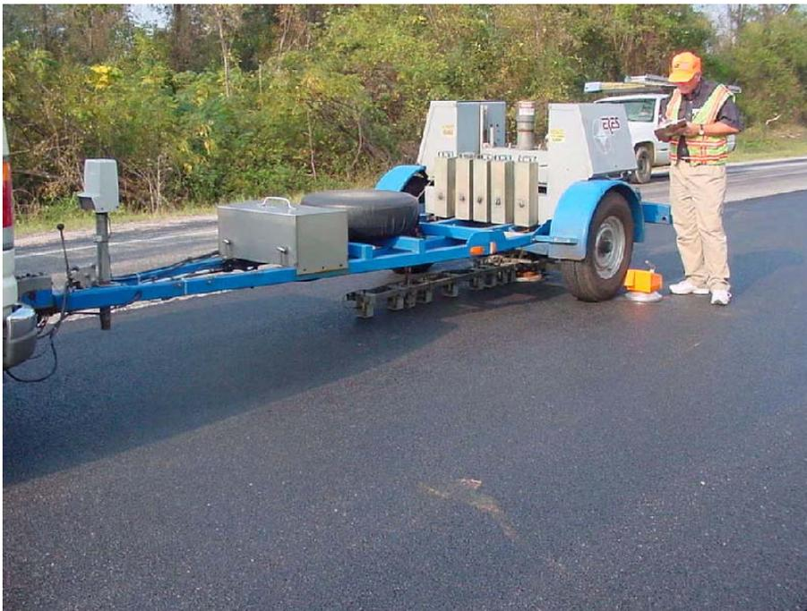
**Figure 28 Falling Weight Deflectometer**
