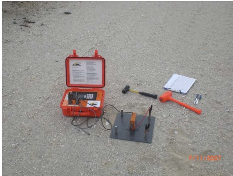
Figure 3.3: Electric Density Gauge Setup
