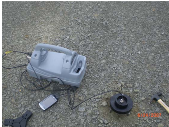
Figure 3.2: Moisture Density Indicator-MDI 2000 Setup
