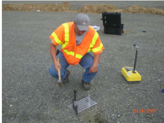
Figure 3.1: Nuclear Gauge Setup
