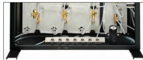
Rear of panel showing quick-connect hookups and plumbing.
