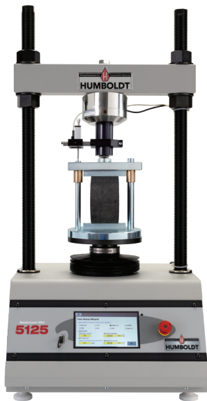
IDEAL-CT (TTI Method) ASTM D8225
