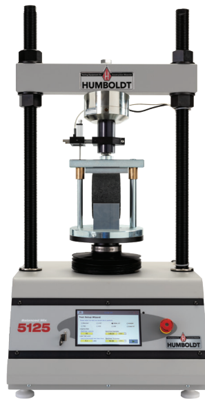
IDEAL-RT (TTI Method) ASTM D8360-22
